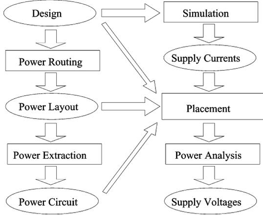
Fig. 3. Flow for evaluating voltage-degradation-aware placement techniques.
