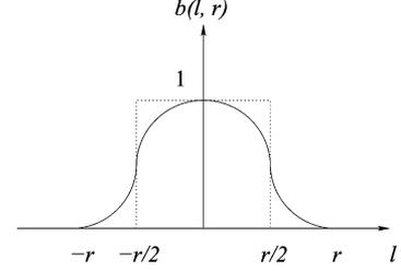
Fig. 2. Bell-shaped function  $b(l, r)$  (in solid curves) which approximates the pulse function (in dotted lines) of width  $r$  and height 1. The areas under the bell-shaped function and the pulse function are equal.
