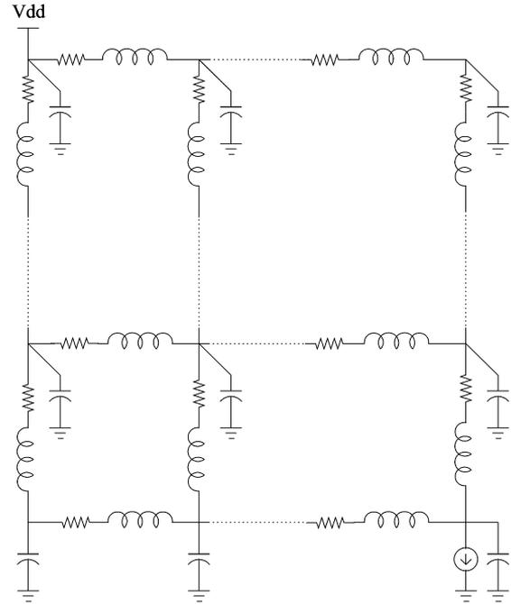
Fig. 1. Power supply grid with a resistor and an inductor on each segment and a ground capacitor and a possible voltage/current source at each node.
