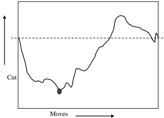
Fig. 2. Characteristic profile of solution cost change during one FM pass. The lowest-cost solution seen during the pass (best prefix of moves) is highlighted; this is adopted as the initial solution for the next pass.
