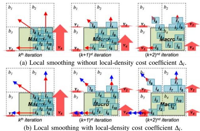
Fig. 2: Local smoothing methods (a) without and (b) with local-density cost coefficient  $\Delta_i$ . Figures are ordered from left to right by iteration indices. Red arrows depict the repulsive force component induced from the  $v_j$ . Blue arrows depict the repulsive force component induced from the local-density cost coefficient  $\Delta_i$ . Figure (b) shows the effect of a larger force to spread cells from the overflowed bin  $b_4$ .
