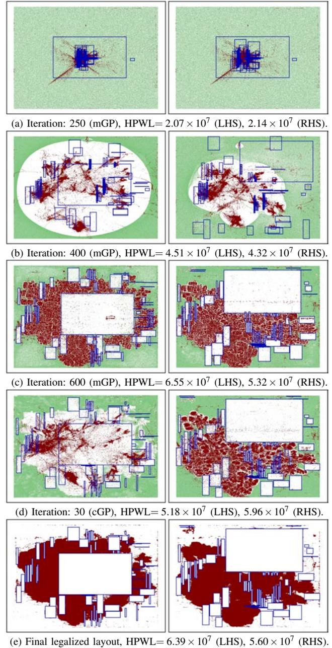
Fig. 3: Placement of *NEWBLUE1* [43]: left hand side (LHS) images are from ePlace-MS [29], and right hand side (RHS) images are from RePIAce-ld. The target density is set to 100%.
