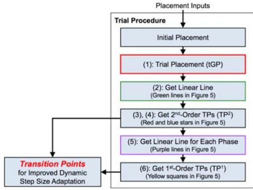
Fig. 6: Flowchart of our trial placement procedure. The red rectangle indicates nonlinear optimization using Nesterov’s method. The actual placement procedure follows this trial placement procedure.
