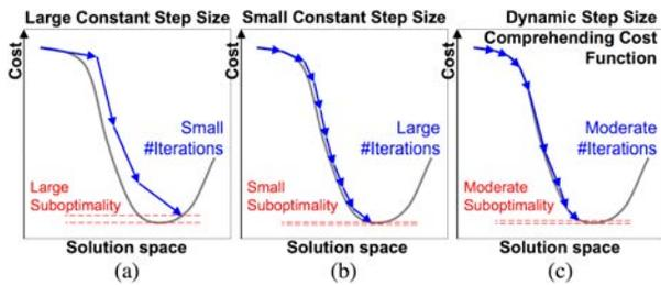
Fig. 4: An illustration conceptually showing the benefit of dynamic step size adaptation. Cost is composite of wirelength and density. (a) Constant large step size obtains a result quickly but with large suboptimality. (b) Constant small step size may generate a near-optimal result but with many iterations. (c) Our improved dynamic step size adaptation starts and ends with small step sizes, and dynamically scales the step size to efficiently allocate the optimization effort.
