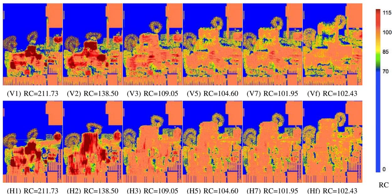
Fig. 10: Global routing overflow (*SUPERBLUE12*) during routability-driven global placement procedure. RC = Routing Congestion reported by the DAC-2012 official evaluation script. (Hk) and (Vk) show horizontal and vertical congestion before the  $k^{th}$  cell inflation; (Hf) and (Vf) show final horizontal and vertical routing congestion after detailed placement.
