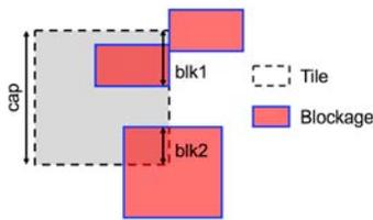
Fig. 8: Illustration of blockage calculation. For the vertical edge on the right,  $blk = blk1 + blk2$ . Note the union of blocked capacity for the upper two blockages.
