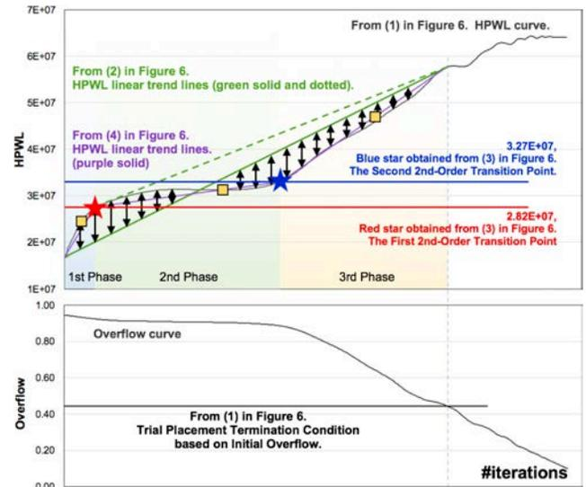
Fig. 5: HPWL curve of *ADAPTECI* from the trial placement procedure and the estimated transition points ( $TP^2$ =red/blue stars,  $TP^1$ =yellow squares).
