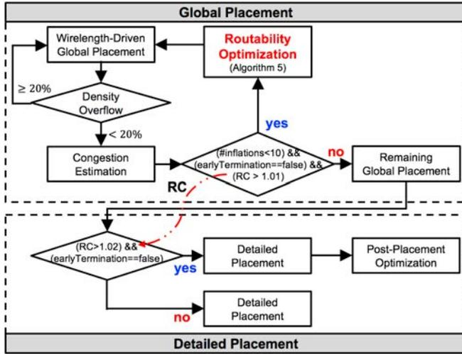
Fig. 9: Overall flowchart of our routability-driven placement.
