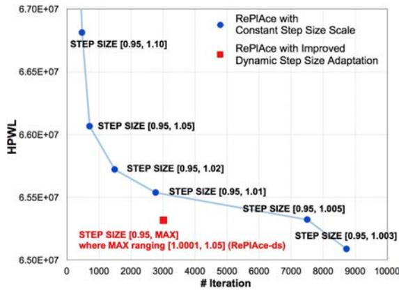
Fig. 7: Solution qualities achieved by RePIAce with constant step size scale and by RePIAce-ds’ improved dynamic step size adaptation strategy, on the *ADAPTECI* [43] testcase. RePIAce-ds achieves a dominating runtime and solution quality (red square). We note that RePIAce with constant step size scale (blue line) does not converge with smaller step sizes (i.e., [0.95, 1.002] or below).
